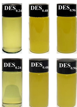
Fig. S1 Photographs of three friction-triggered self-reactive DESs samples before and after vacuum drying. The top row shows the samples before drying, and the bottom
