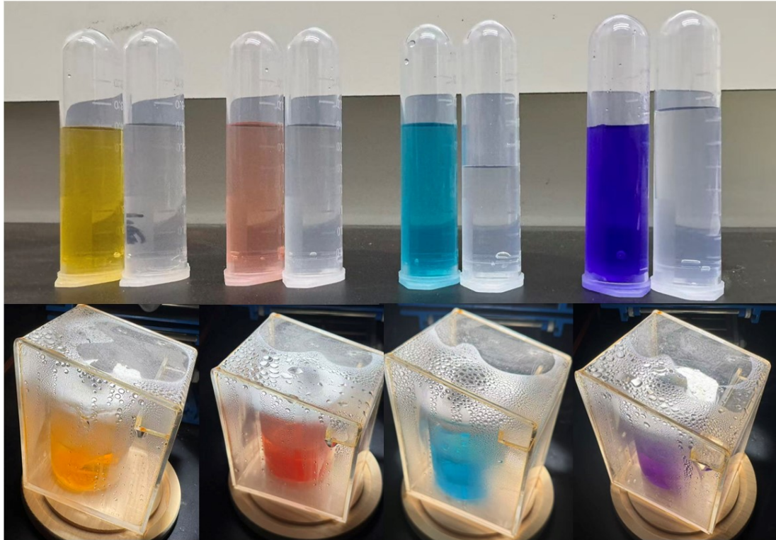
Figure S15. The decolorization experiments of FCSC for organic dyes.
