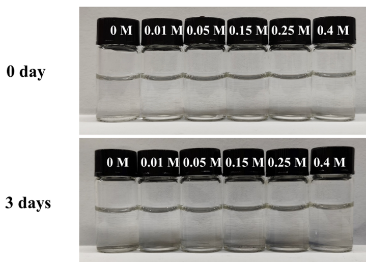
Figure S2. Optical photographs of ZSO electrolytes containing various molar mass of SPE additives (0 M, 0.01 M, 0.05 M, 0.15 M, 0.25 M, 0.4 M).
