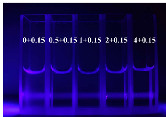
Figure S4. Tyndall Effect of 0.15 M SPE in ZnSO 4 Solutions with different concentrations.
