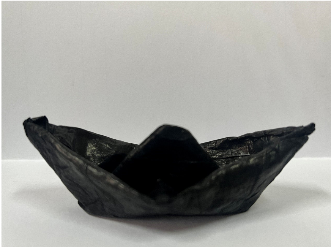
Fig.S8 The carbon nanotube film is folded into a boat.
