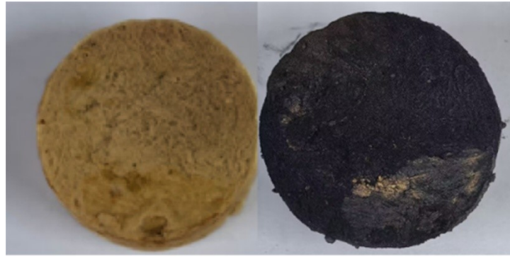
Fig. S21 Digital photos of BCPA100 aerogel before and after butane torch flame test.
