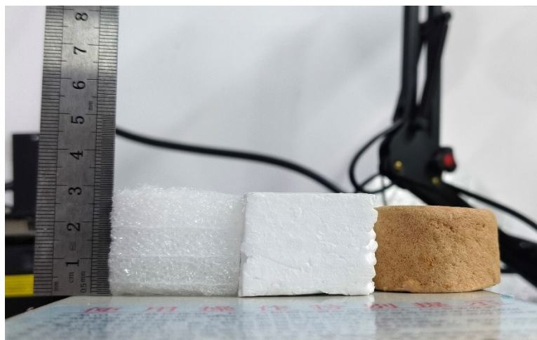
Fig. S16 Digital photos of EPE foam (left), EPE foam (middle) and BCPA100 aerogel (right) for thermal insulation test.
