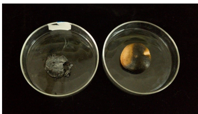
Fig. S18 Digital photos of BCA15 aerogel (left) and BCPA100 aerogel (right) after burning over an alcohol lamp.
