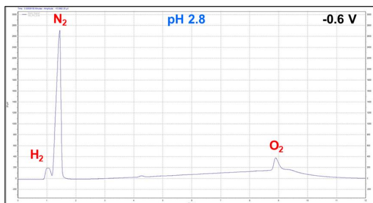
Figure S15. GC (TCD) chromatogram obtained for the electrochemical eNO 3 RR performed with ZnWO 4 in acetate buffer (0.2 M, pH 2.8) at -0.6 V vs. RHE in a closed container using the three-electrode setup (WE: \alpha -SnWO 4 loaded on CC, RE: Ag/AgCl (aq.), and CE: graphite rod).
