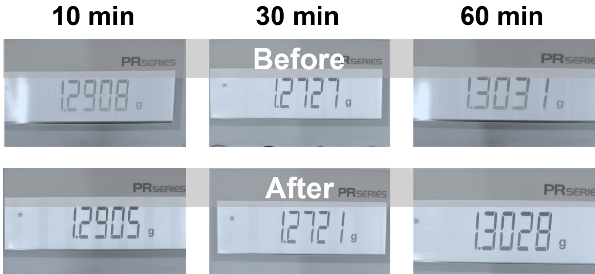
Figure S6 The mass losses of BTT evaporator after ultrasonication. Due to the uneven voids of FT, the initial weights of the BTT evaporators are inconsistent. BTT evaporators were immersed in deionized water and subjected to ultrasonication for different durations (10, 30, and 60 min).
