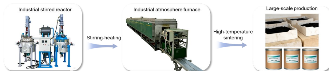
Fig. S43: Industrial-Scale Preparation Engineering. Cotton fiber feedstock and MSA were first added into a large-scale corrosion-resistant industrial stirred reactor for mixing. The system was heated to 80°C; upon reaction completion, the mixture was separated (solid-liquid) and transferred to a large-scale industrial atmosphere sintering furnace. Under flowing argon, the furnace was heated to 1300°C, held isothermally for 3 h, and cooled naturally to yield kilogram-scale HC.
