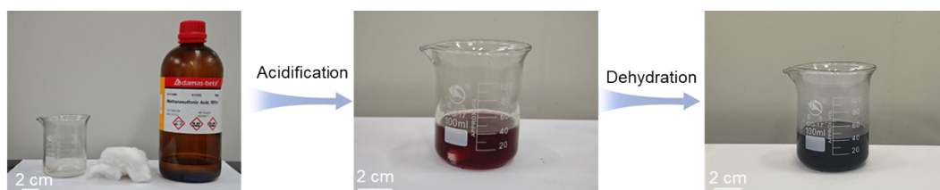
Fig. S1: Flow chart for the methanesulfonic acid treatment of biomass. Acidolysis of cotton in MSA generates molecules with extended conjugated systems, imparting a purple color to the solution. Subsequent deep dehydration of the cotton into carbonaceous material results in a color change of the solution to black.
