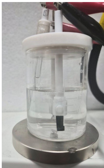
Fig. S8 Electrochemical cell set up with magnet.
