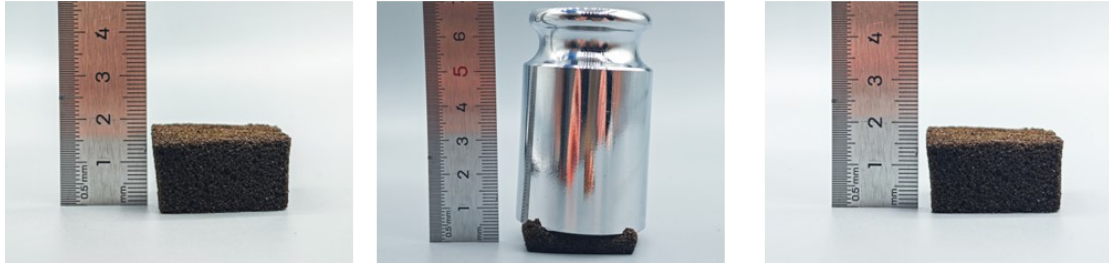
Figure S7. Photographs of the LEH before, during, and after a static compression test under a 500 g weight for 10 min.
