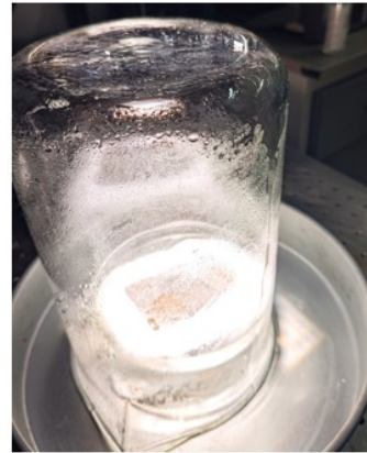
Figure S17. Condensate collection setup for module-assisted freshwater generation: (a) photograph of LEH coupled with the auxiliary water module, (b) photograph of the condensate collection device, and (c) water vapor condensation on the inner wall during operation.
