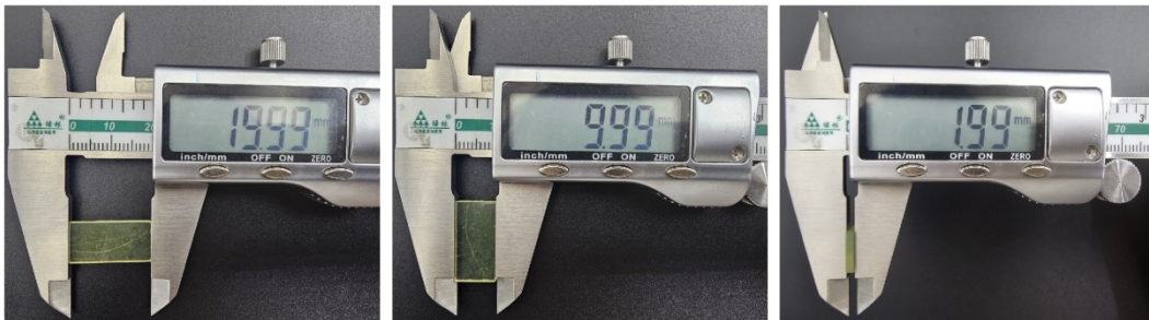
Figure S3. Dimensions of the printed specimens ( 20 \times 10 \times 2 mm) under different curing conditions: (A) immediately after printing, (B) after storage in the dark for 3 h, and (C) after 30 min of UV post-curing.
