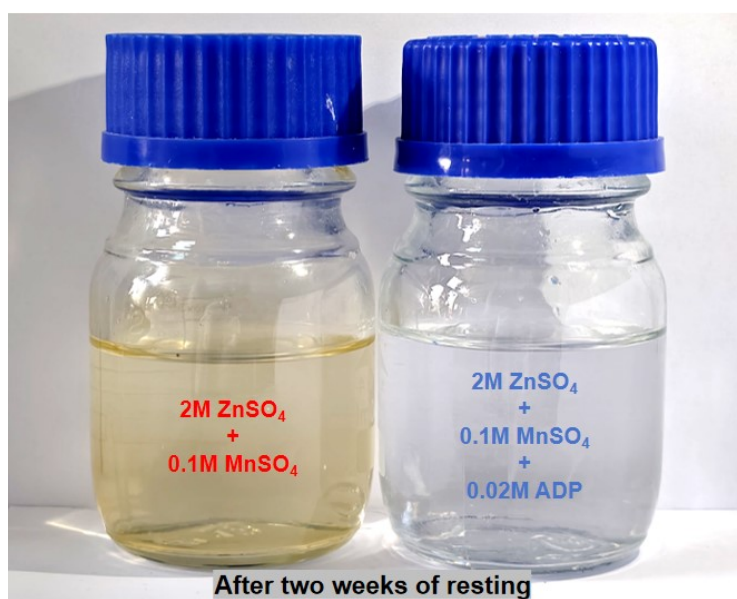
Fig. S30 Electrolyte storage test. Digital photographs of electrolytes after resting for two weeks. The standard electrolyte turns yellow, whereas the ADP-containing electrolyte remains relatively clear, suggesting improved electrolyte storage stability.
