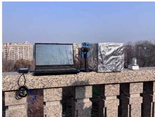
Fig. S11 Photograph of a homemade outdoor radiative cooling performance testing apparatus.
