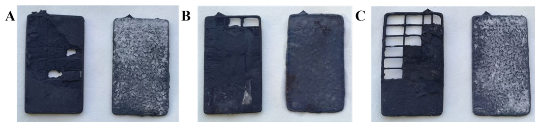
Fig. S6. Photographs of the positive electrode (left) and negative electrode (right) after cycling: (A) Blank battery, (B) RHAC battery, (C) PbO/RHAC battery.
