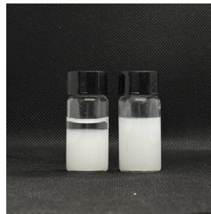
Figure S1. Stability of C-S-H suspension with (right) and without (left) PVA manipulation indicating the inhibited agglomeration of C-S-H
