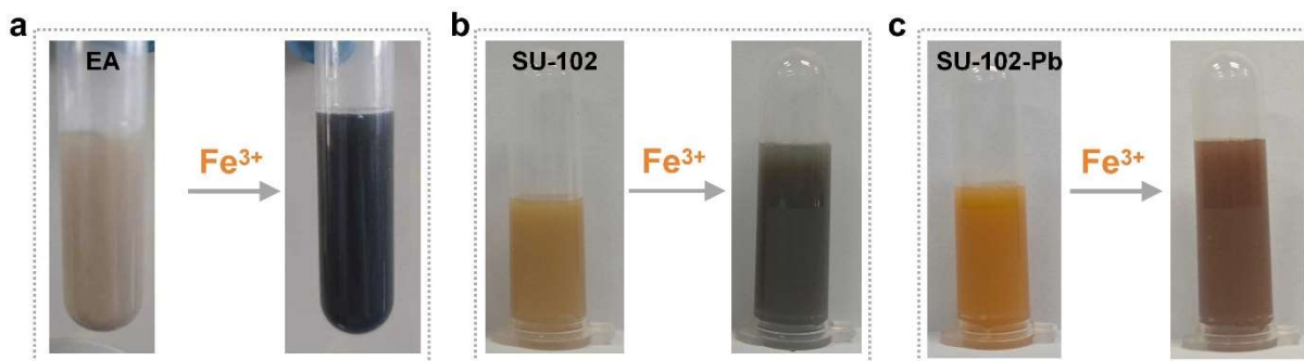
Fig. S5. Optical photos of color changes before and after introducing \text{Fe}^{3+} into EA, SU-102, and SU-102-Pb suspensions, respectively.
