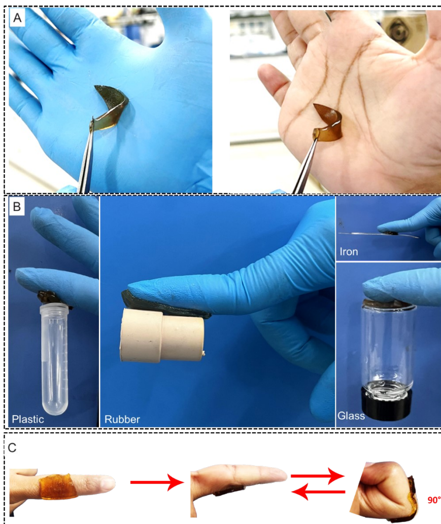
Fig. S6 (A) Hydrogels adhered to hands both with and without glove which can be peeled off without leaving any residue. (B) Hydrogels adhered to various organic and inorganic surfaces. (C) Adhesive behavior of PAM/Ag@HA hydrogel on finger joint.
