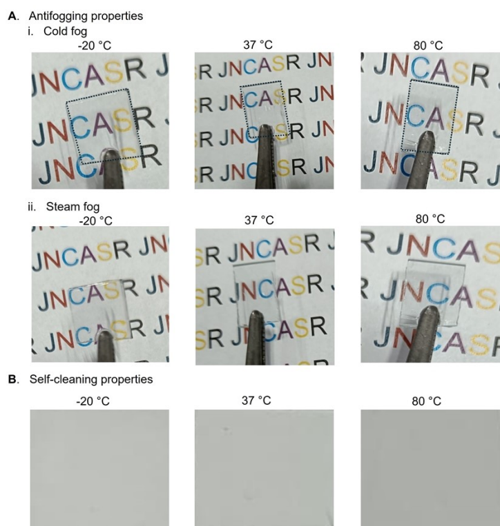
Figure S7: Digital image of (A) antifogging property; (B) self-cleaning properties of GDQP pr -10 surfaces after exposure to different temperatures: -20 °C, 37 °C, and 80 °C.
