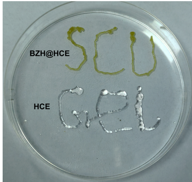
Figure S3. Injectability testing demonstrated that the hydrogel could be smoothly extruded through syringe needle (0.5 mm inner diameter) and maintain its structural integrity after extrusion.
