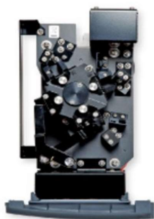
ISR-2600Plus Integrating Sphere Attachment
