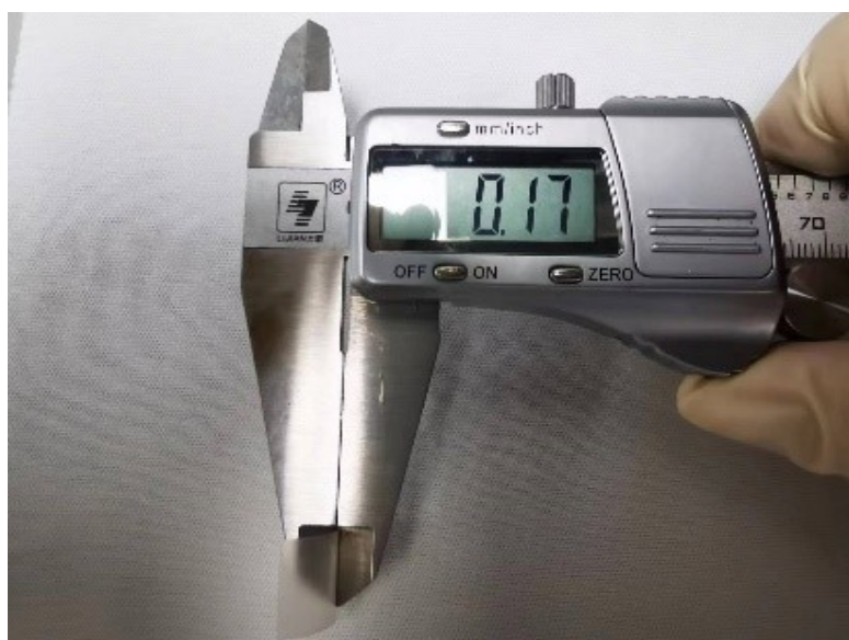
Supplementary Figure 2. Thickness measurement of TPU-IL-ZnO-SiO 2 film.
