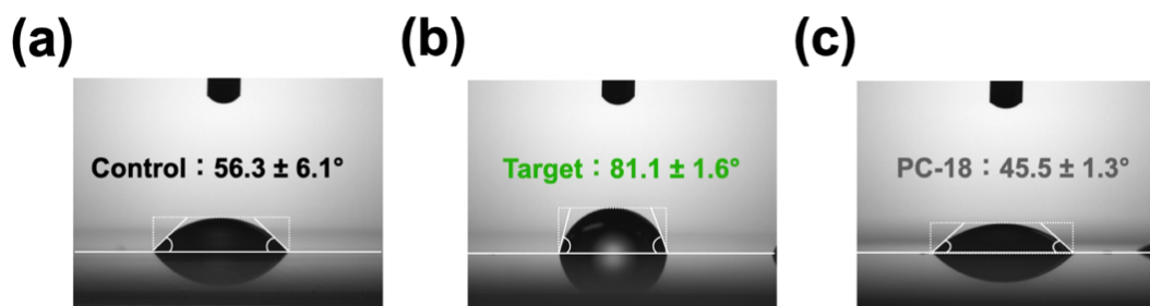
Fig. S12 Contact angle measurements of spin-coated PeNC thin films: (a) Control, (b) Target, and (c) Octadecylphosphocholine (PC-18)—treated samples
