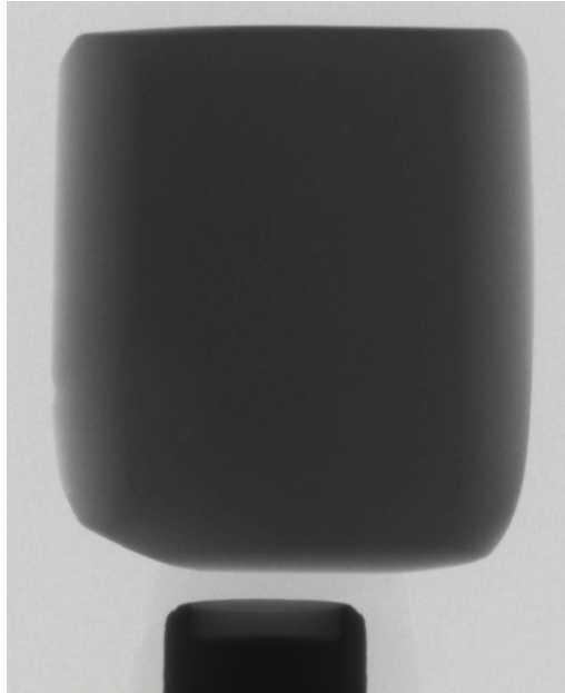
23 Figure S2. X-ray transmission image of the SGMC containing 1 wt.% of SMSO.
