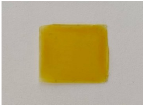
Fig. S27. PS- b -PPI membrane picture of formed by poly( 1_{200} - b - 2L_{100} ). Films were prepared by solvent casting from a polymer solution in a PTFE mold.
