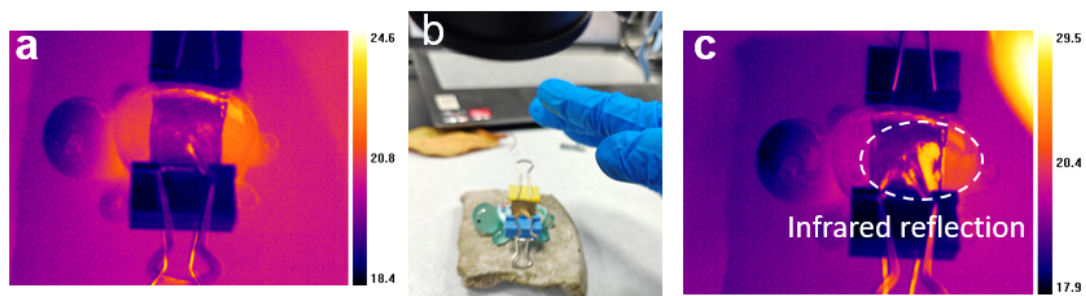
Figure S10. Simulating proximity to a heat source with the palm, infrared reflection occurs on the Au side.
