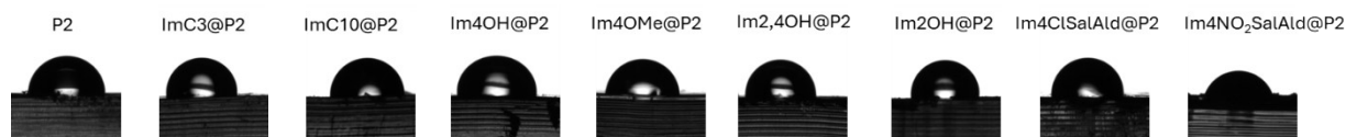
Fotos: S19: Static contact angle images of water at the photopolymer surface of P2 coated with C3 = propionaldehyde C10 = decan aldehyde, 4OH = 4-hydroxybenzaldehyde, 4OMe = 4methoxybenzaldehyde, 2,4OH = 2,4dihydroxybenzaldehyde, 2OH = 2 hydroxybenzaldehyde, 4Cl2OH = 4 chloro-2 hydroxybenzaldehyde, 4NO 2 2OH = 4 nitro 2 hydroxybenzaldehyde.
