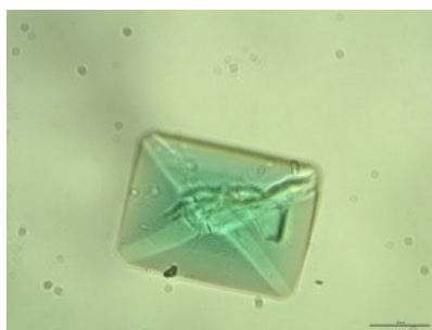
Figure S2. Optical images of the as-synthesized ZJU-132. Scale bar: 50 \mu\text{m} .
