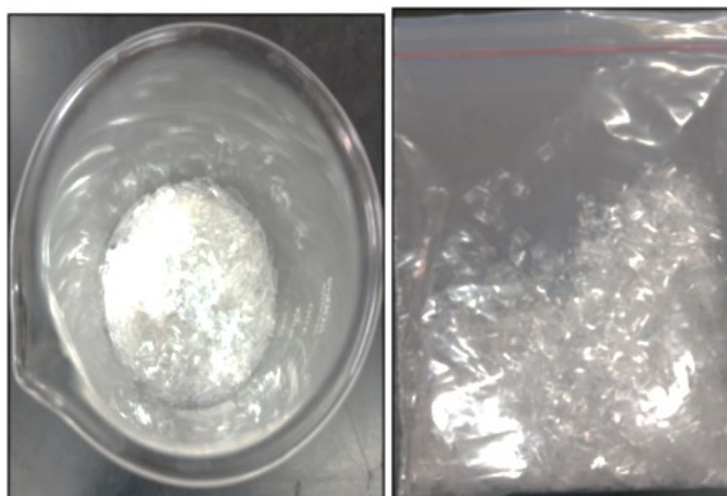
Fig S1: PET bottle waste in crushed form serves as the raw material for producing carbon dots.
