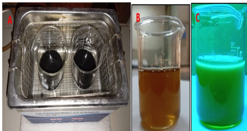
Fig S3: Sonication process for synthesizing carbon dots (A), their dispersion seen under daylight (B), and the characteristic green fluorescence of carbon dots under UV light (C)
