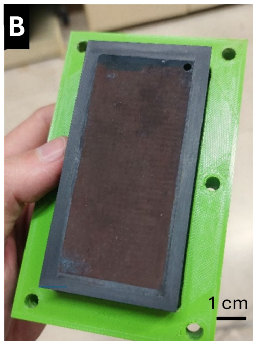
Figure S1. (A) LMO electrode deposited on the current collector before oxidation. (B) LMO electrode after the oxidation process, with a noticeable reddish color on the surface in contact with the solution.
