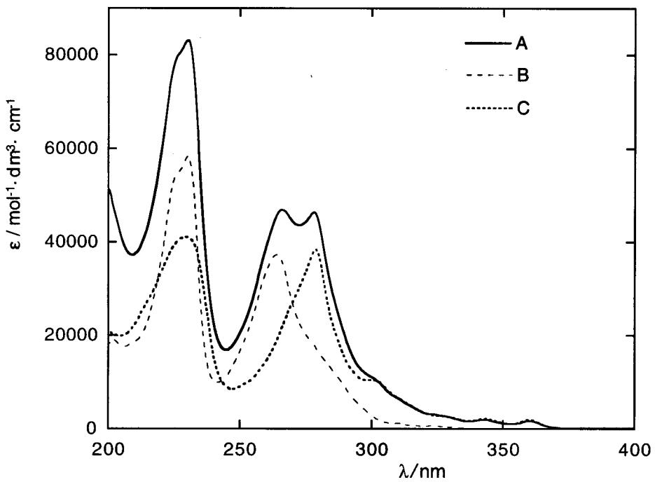
Fig. S2. UV-Vis absorption spectra of: (A)  $[\text{Pt}(\text{en})(\text{phen})](\text{PF}_6)_2 \cdot \text{phen} \cdot 2\text{H}_2\text{O}$ , (B) free phen, (c)  $[\text{Pt}(\text{en})(\text{phen})](\text{PF}_6)_2$  in EtOH/MeOH(4:1 v/v).
