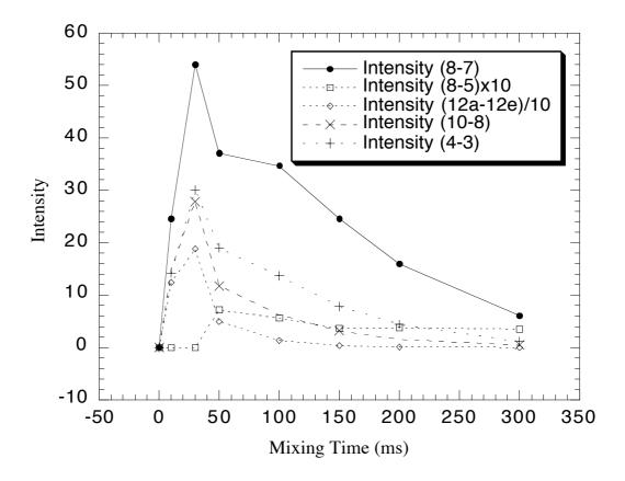
**Figure S2:** ROE build-up line plots for cross-peaks for 25 mM a-phi. Five representative protons are chosen to show that no evidence of spin diffusion is seen before a mixing time of 50 ms.
