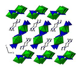
Figure S2. Three-dimensional packing of USO-7. Blue tetrahedra and green pentagonal bipyramids represent  $[SO_4]$  and  $[UO_7]$  respectively. Blue and white circles represent nitrogen and carbon atoms. Hydrogen atoms have been removed for clarity.
