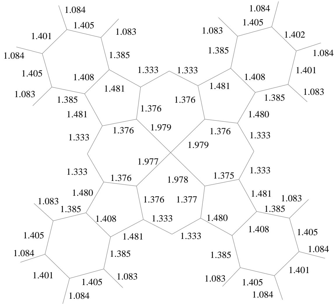
(Electronic Supplementary Information) Figure 2. Optimized geometry of LiPc. Bond length in angstrom.
