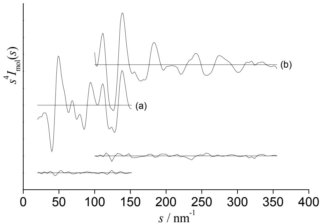
**Figure S2.** Molecular scattering intensity and final weighted difference curves for hexasilylbenzene. (a) Long camera distance. (b) Short camera distance.
