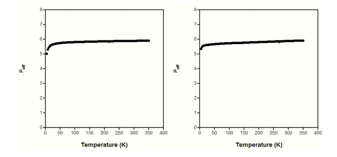
**Figure S2.** Temperature dependent magnetic moment (10 kG) of [Fe(3,2-HOPTO)<sub>3</sub>] (left) and [Fe(3,4-HOPTO)<sub>3</sub>] (right).
