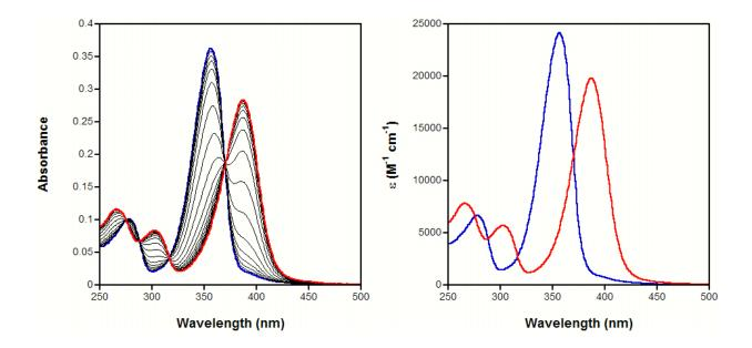
**Figure S3.** Experimental spectra (left) from a representative spectrophotometric titration of thiomaltol. The initial (low pH) spectrum is shown in blue and the final (high pH) spectrum is shown in red (I = 0.1 KCl; T = 25 °C). Calculated spectra (right) from factor analysis for protonated (blue) and deprotonated (red) thiomaltol.
