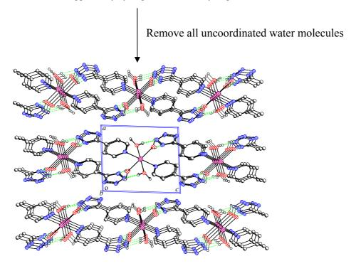
Three layers of two-dimensional framework consisting of [Mn $\{5-(4-pyridyl)-tetrazolato\}_2(H_2O)_4$ ] units linked by 'intermolecule' hydrogen bonds
