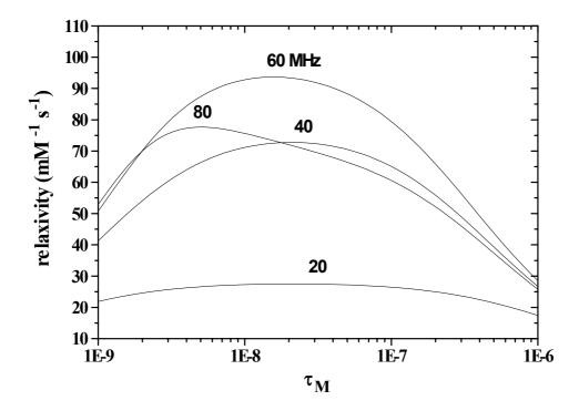
The figure shows a simulation of the effect of altering  $\tau_M$  on relaxivity at four different magnetic fields for a gadolinium chelate with retricted rotation. It is apparent that as the magnetic field increases so the maximum relaxivity is achieved with increasingly short  $\tau_M$  values. A value of tM of 6 ns as exhibited by GdS-SSS-NO<sub>2</sub>BnDO3MA-1A seems likely to be a particularly effect value at magnetic fields in the region of 100 MHz.
