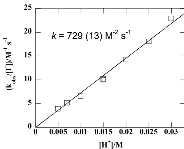
**Figure S5.** Plot of  $k_{\text{obs}}/[\text{I}]$  vs  $[\text{H}^+]$  for the reaction of  $\text{L}^2(\text{H}_2\text{O})\text{CrOO}^{2+}$  with  $\text{I}^-$ .
