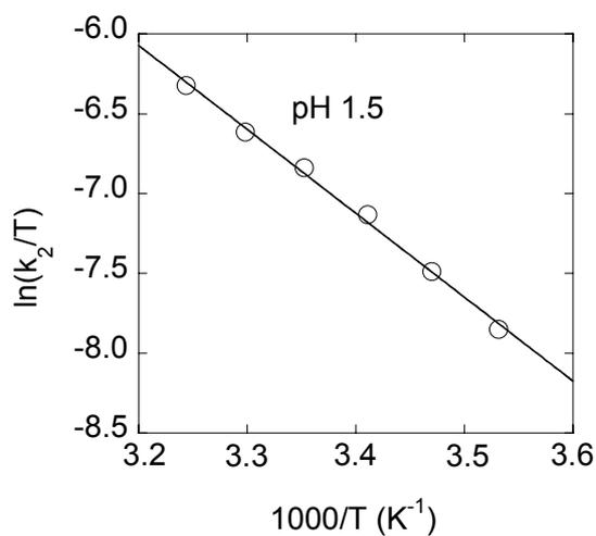
**Figure S3.** Plots of  $\ln(k_2/T)$  vs  $1/T$  for the decay of  $L^2Cr(V)$ .
