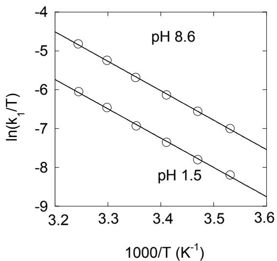
**Figure S2.** Plot of  $\ln(k_1/T)$  vs  $1/T$  for the formation of  $\text{L}^2\text{Cr}(\text{V})$ .
