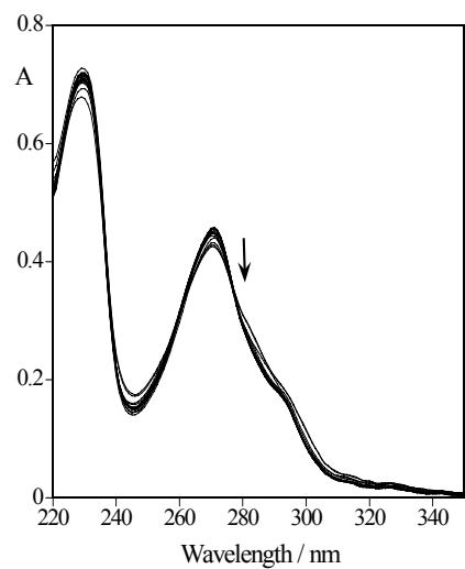
**Fig. S2.** pH dependence of the absorption spectra of L1 aqueous solution. (  $[L1] = 1.30 \cdot 10^{-5}$  M I = 0.1 M NMe<sub>4</sub>Cl, 298 K). (pH = 1.16; 1.51; 1.73; 2.07; 2.28; 2.50; 2.76; 3.07; 3.60; 4.05; 4.72; 5.30; 6.00; 6.22; 6.39; 6.77; 7.30; 8.25; 9.11; 10.78; 11.30).
