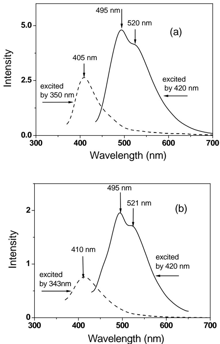
**Figure S1.** Fluorescence emission spectra at 293 K in DMSO-H<sub>2</sub>O (80:20) (a) QB1 ( $1.0 \times 10^{-4}$  mol/L) only and zinc perchlorate ( $2.0 \times 10^{-3}$  mol/L) was added, respectively. (b) QB2 ( $1.0 \times 10^{-5}$  mol/L) only and zinc perchlorate ( $1.5 \times 10^{-4}$  mol/L) was added, respectively. The dashed line corresponds to the free chemosensors only and the solid line to the zinc complexes.
