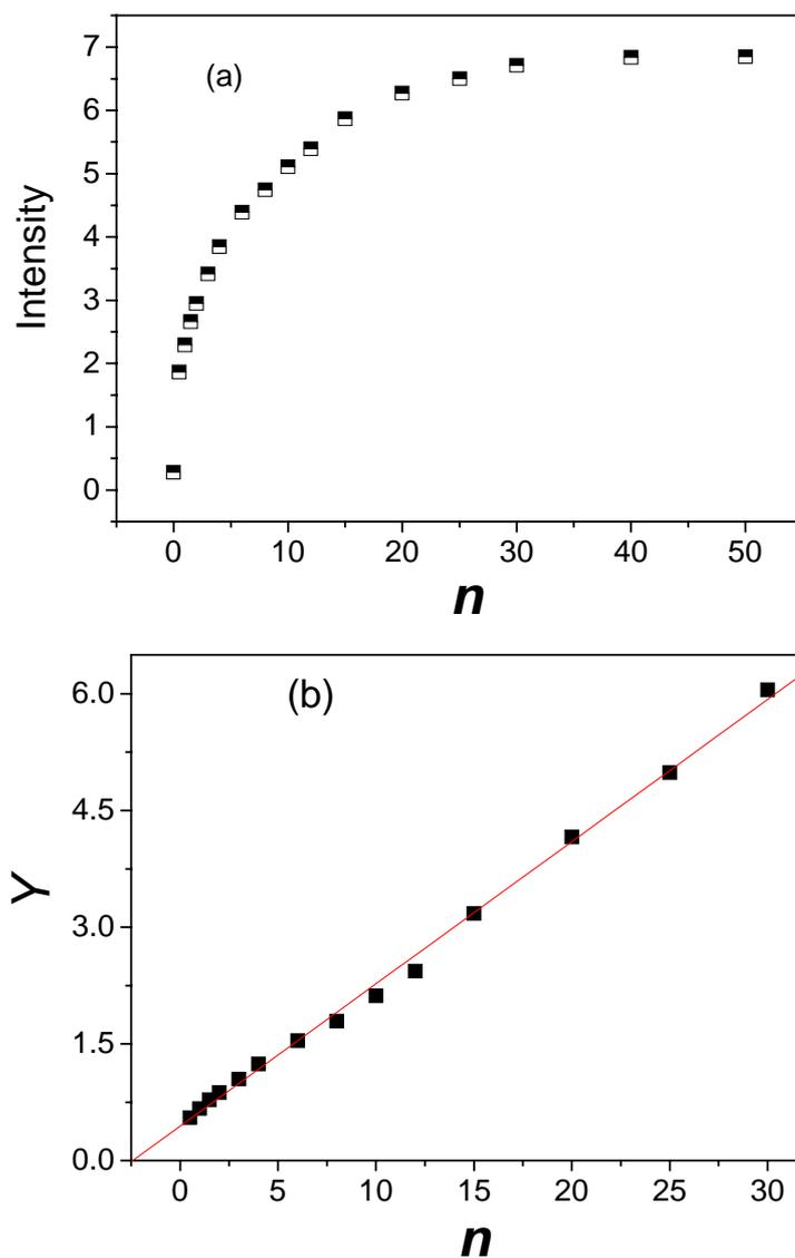
**Figure S3.** (a) Fluorescent intensity changes at 495 nm vs the equivalent molar ratio of  $\text{Zn}^{2+}$  added (Excitation wavelength at 420 nm with the concentration of QB1 being  $1.0 \times 10^{-4} \text{M}$ ). (b) Plot for QB1- $\text{Zn}^{2+}$  system with  $K_{ass}$  being calculated as  $4.08 \times 10^9 \text{M}^{-3}$ .
