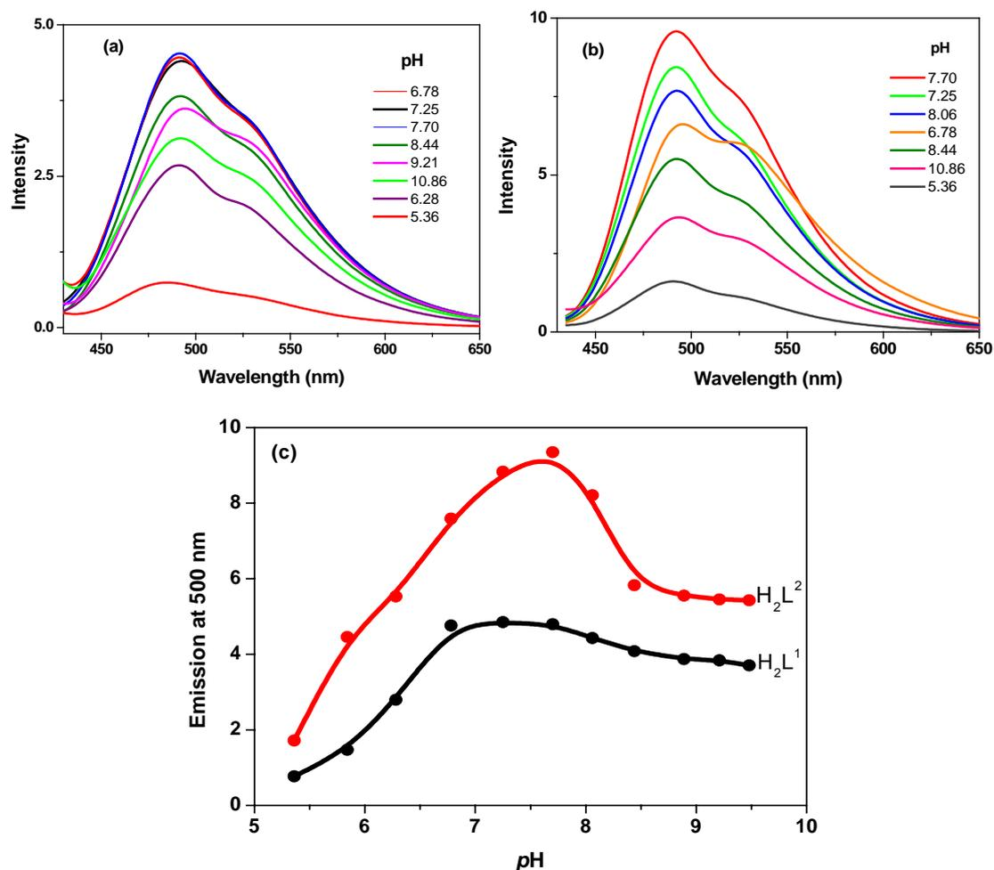
**Figure S6.** Changes in the emission spectra of (a) QB1 (50 μM) (b) QB2 (50 μM) against different pH (HEPES buffer or TRIS buffer) in DMSO – H<sub>2</sub>O (v:v, 40:60) solutions upon addition of Zn(ClO<sub>4</sub>)<sub>2</sub> · 6 H<sub>2</sub>O (0.75 mM) in water. (c) Emission intensity variations of QB with different pH after addition of Zn<sup>2+</sup>, monitored at 420 nm.
