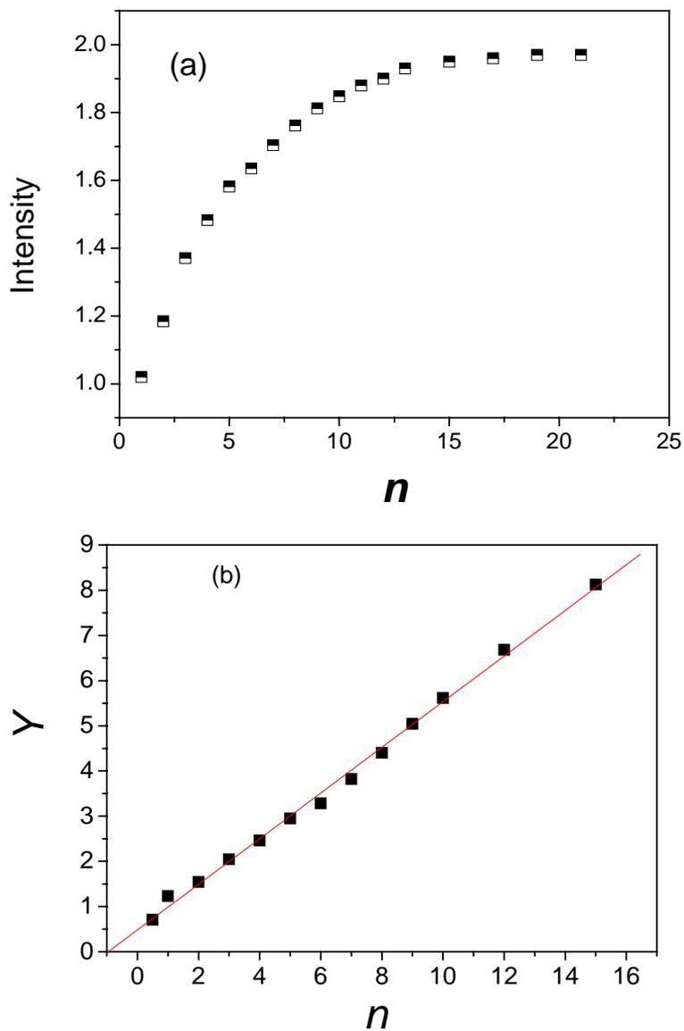
**Figure S4.** (a) Fluorescent intensity changes at 495 nm vs the equivalent molar ratio of  $\text{Zn}^{2+}$  added (Excitation wavelength at 420 nm with the concentration of QB2 being  $1.0 \times 10^{-5} \text{M}$ ). (b) Plot for QB2- $\text{Zn}^{2+}$  system with  $K_{ass}$  being calculated as  $1.27 \times 10^{14} \text{M}^{-3}$ .
