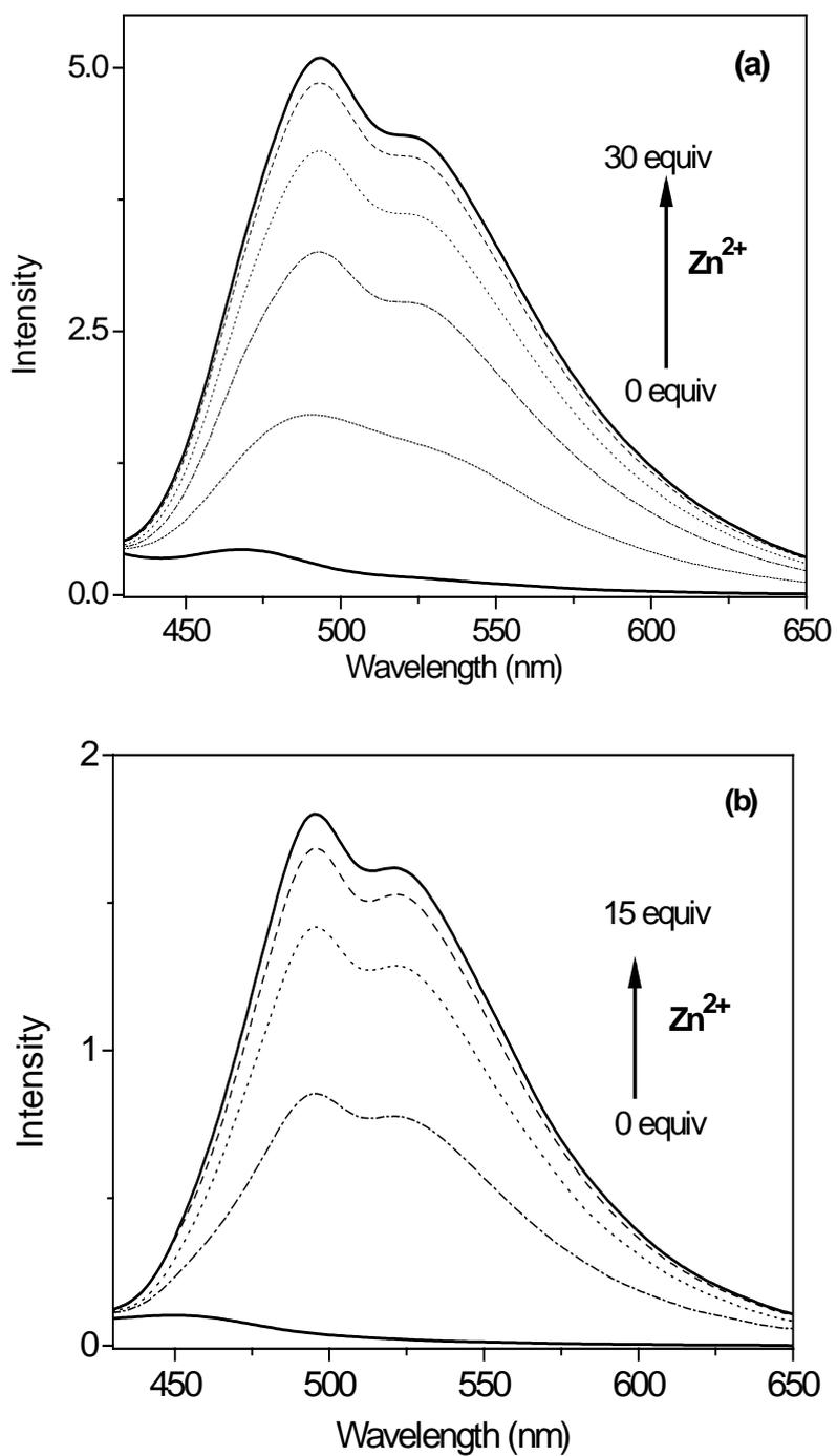
**Figure S2.** Luminescent titrations of receptors QB1 at  $1.0 \times 10^{-4}$  mol/L (a) and QB2 at  $1.0 \times 10^{-5}$  mol/L (b) with increasing concentration of  $Zn^{2+}$ . Excitation wavelength was 420 nm with 4 nm slit widths, and spectra were corrected.
