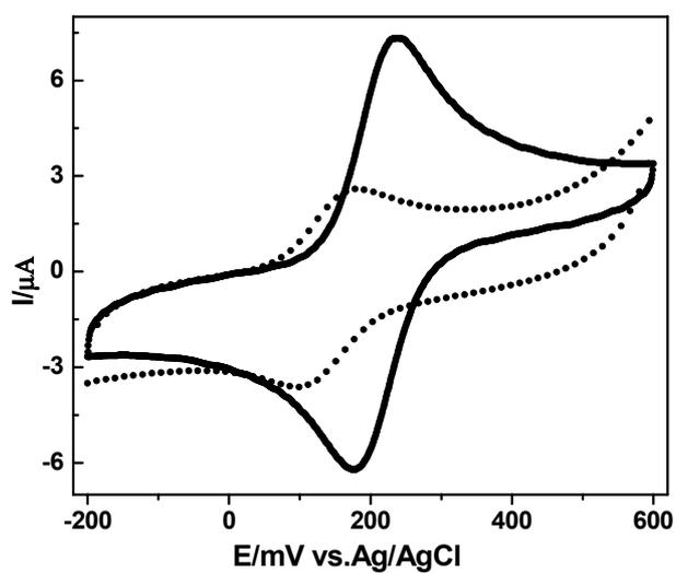
Cyclic voltammogram of 1.0 mM compound 3 (—) and 0.5 mM  $TU^{Fc}T$  trimer (····) in 0.2 M  $NaClO_4$  in  $H_2O$ .
