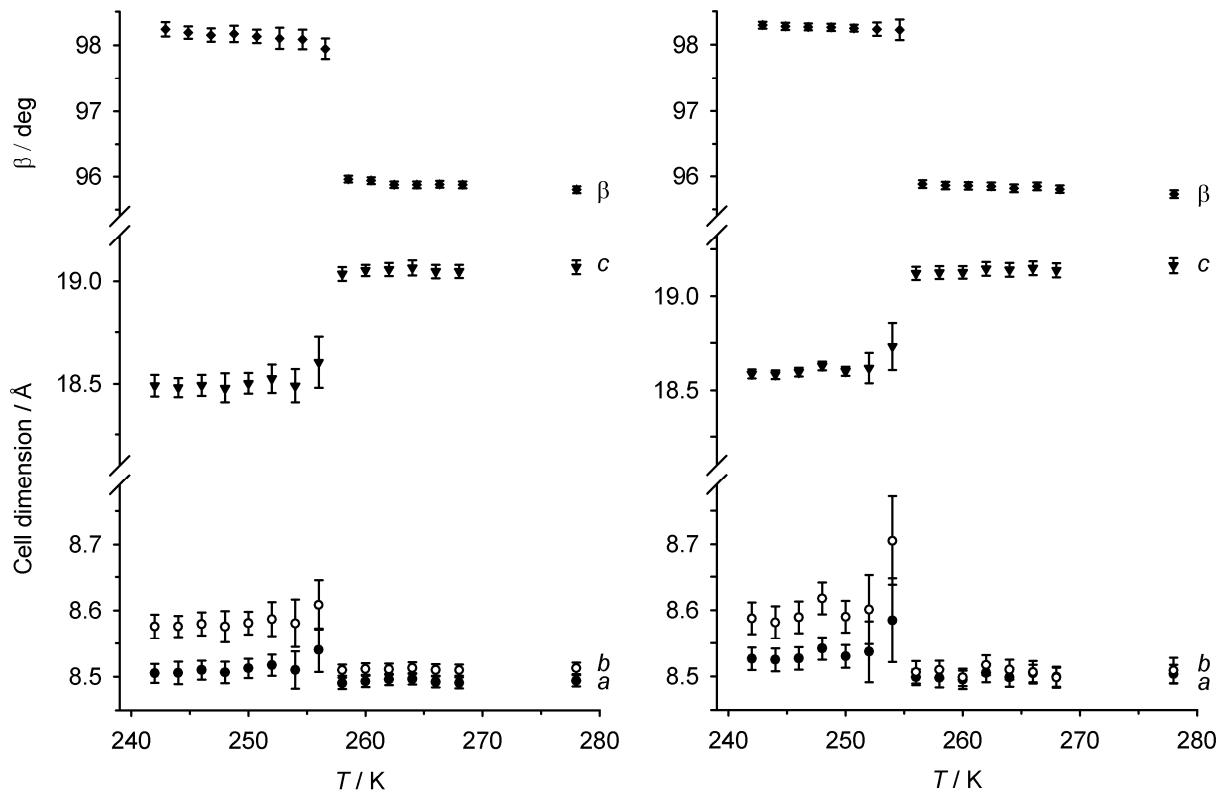
**Figure S2** Variable temperature unit cell dimensions from single crystals of **2** (left) and **3** (right), near their spin-transition temperatures. Corresponding data for **1** are presented in ref. 2.
