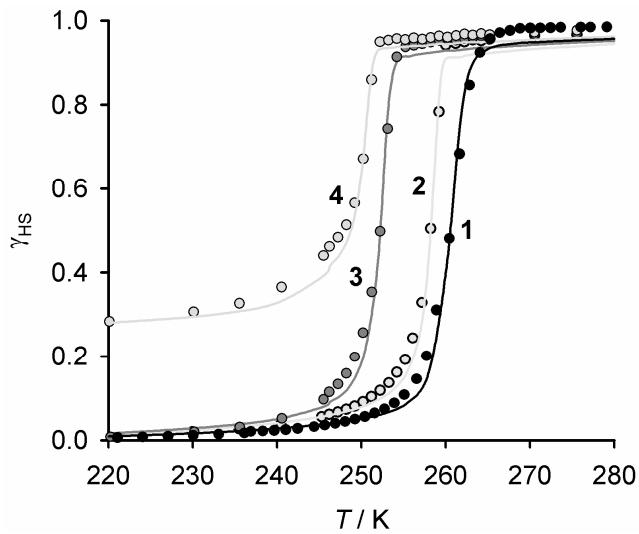
**Figure S1.** Observed (points) and simulated (line) magnetic data for the powder samples of **1-4** in warming mode, using the Slichter and Drickhamer model of solid state phase transitions.<sup>1</sup>  $\gamma_{HS}$  is the high-spin fraction of the sample at a given temperature. The values of the interaction energy  $\Gamma$  derived by this analysis are listed in Table 1 of the main paper.
