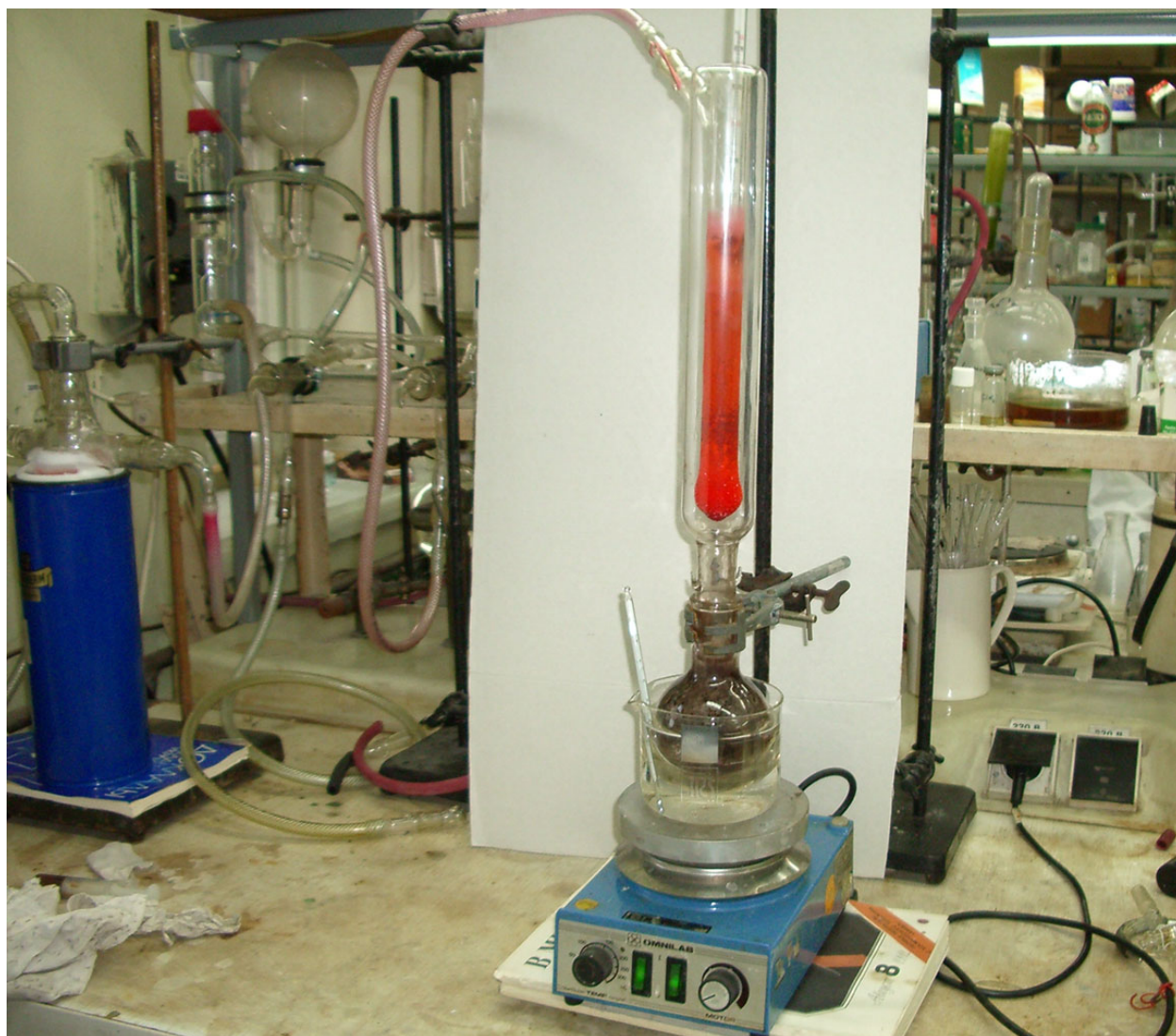
Figure S1. Final step of 1,2,4,5-tetrazine preparation: The foto demonstrates a very simple equipment for isolation of pure tetrazine (in a 10-15 g scale) by direct sublimation at room temperature of the residue after evaporation of the solvent. As a cooling finger we have employed a usual 60 cm adapter for condensation of liquid ammonia, charged with
