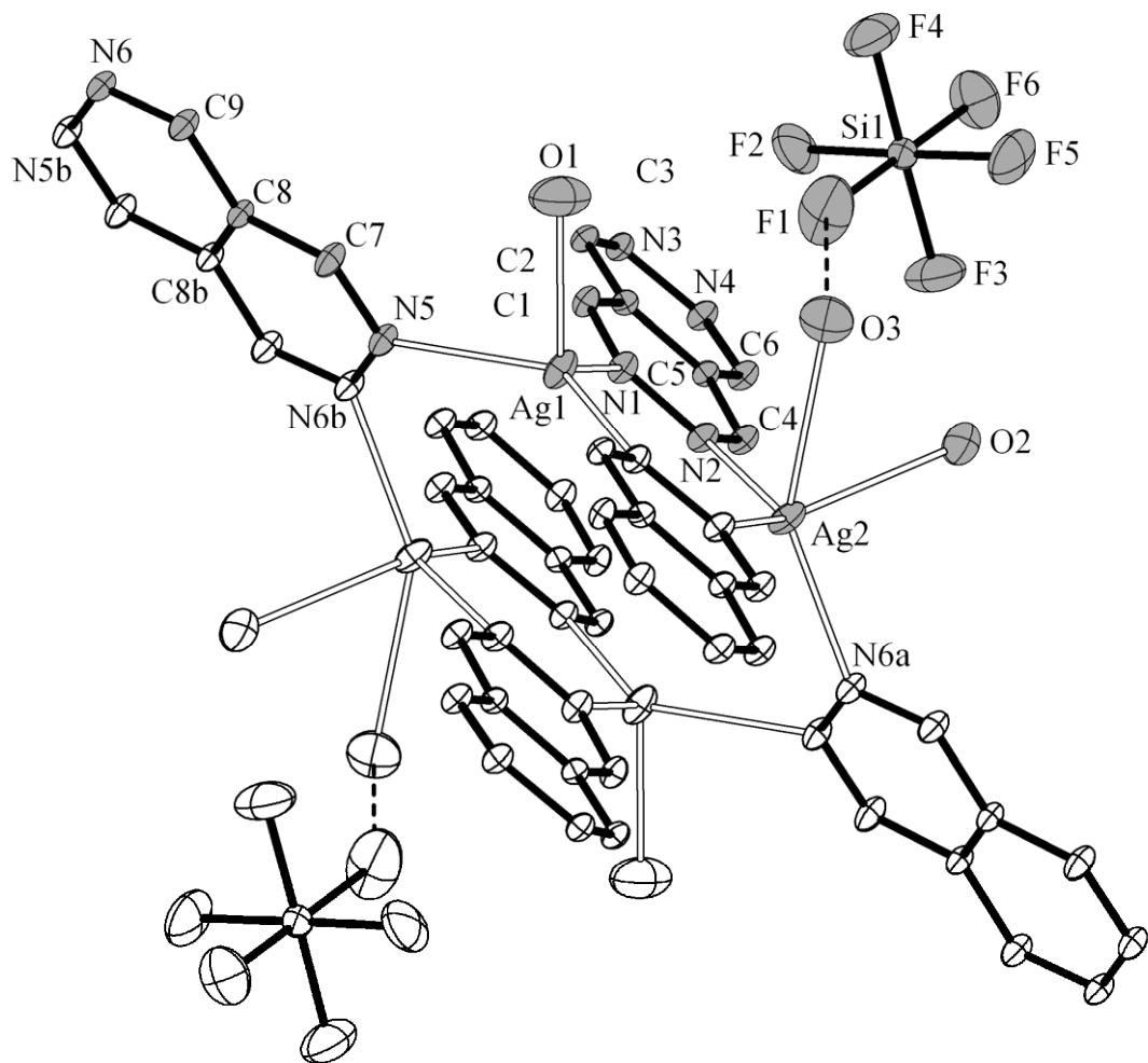
**Figure S5.** ORTEP diagram for  $\text{Ag}_4(pp)_3(\text{SiF}_6)_2 \cdot 10\text{H}_2\text{O}$  (**4**) showing atom labeling scheme.
