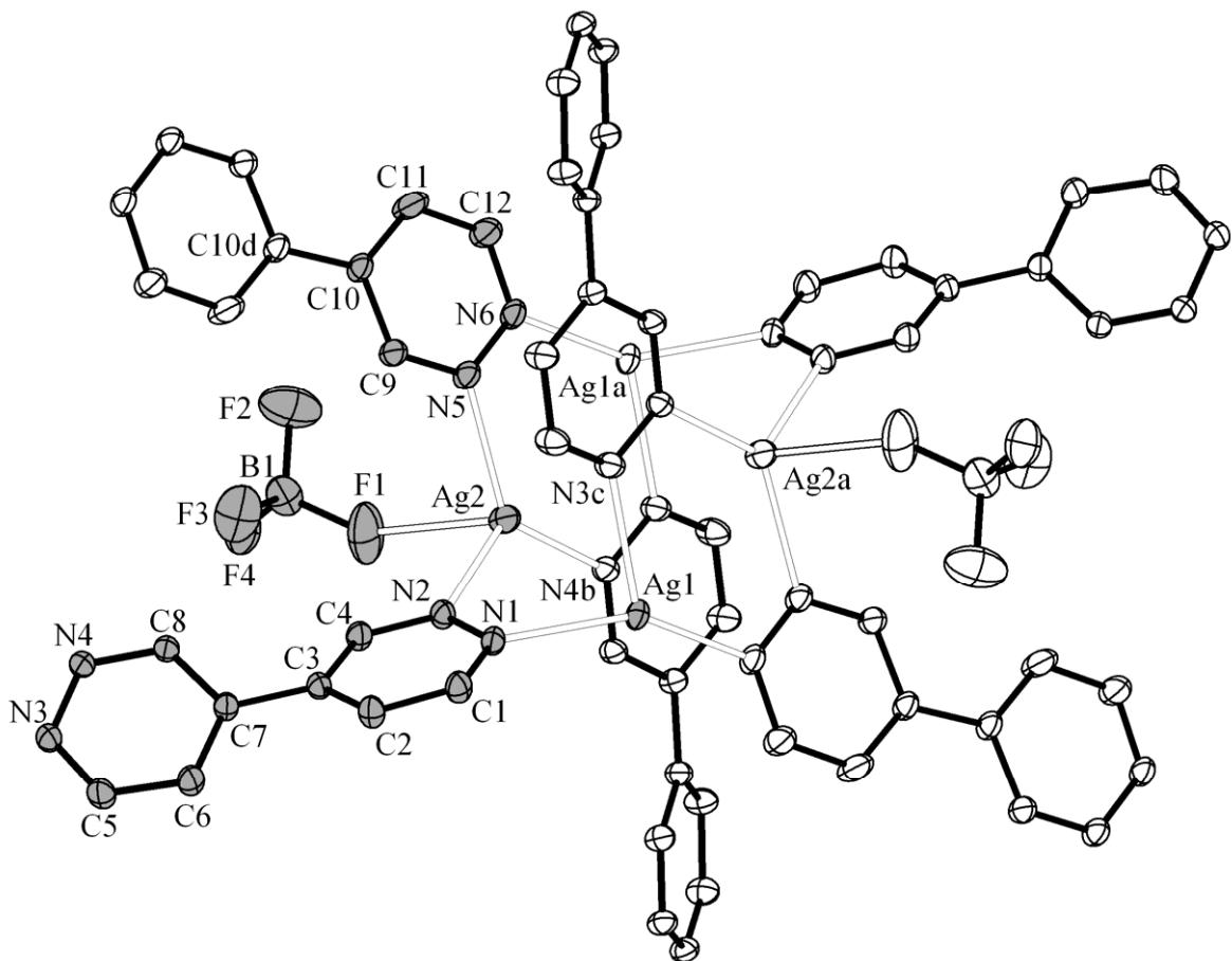
**Figure S8.** ORTEP diagram for  $\text{Ag}_4(\text{bpdz})_3(\text{BF}_4)_4 \cdot \text{H}_2\text{O}$  (**7**) showing atom labeling scheme.
