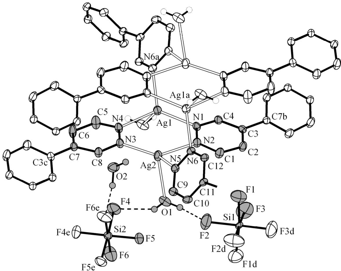
**Figure S9.** ORTEP diagram for  $\text{Ag}_4(\text{bpdz})_3(\text{SiF}_6)_2 \cdot 3\text{H}_2\text{O}$  (**8**) showing atom labeling scheme.
