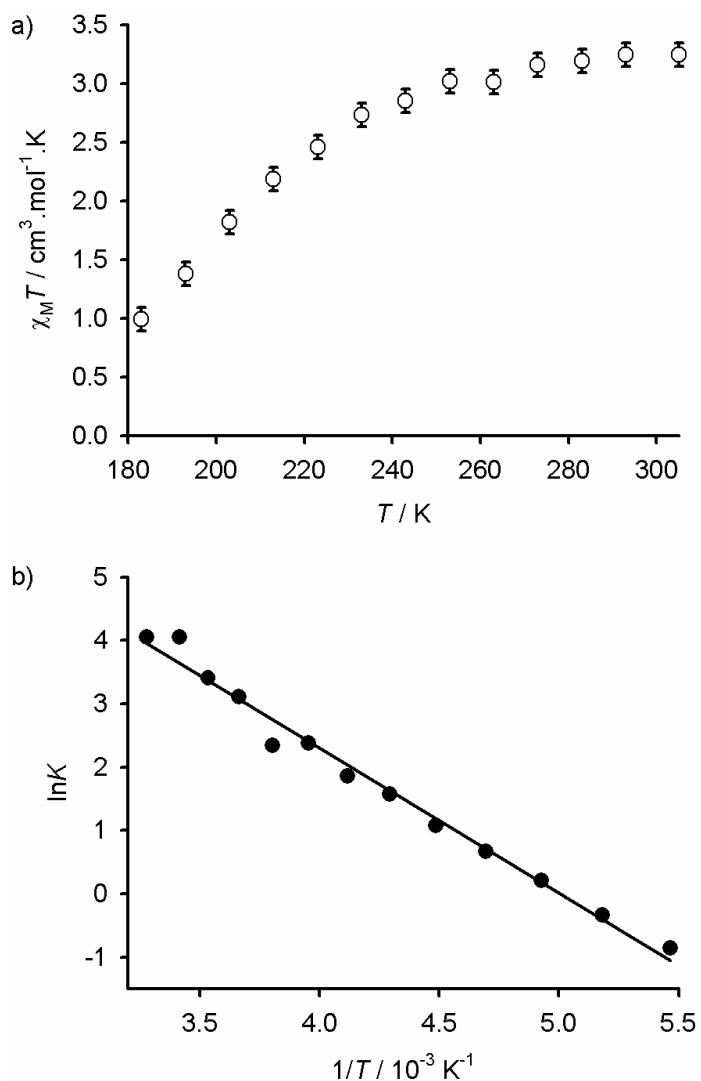
**Figure S5** (a) Plot of  $\chi_M T$  vs.  $T$  for **1**[CF<sub>3</sub>SO<sub>3</sub>]<sub>2</sub> in (CD<sub>3</sub>)<sub>2</sub>CO. (b) van't Hoff isochore plot of the spin-state equilibrium for **1**[CF<sub>3</sub>SO<sub>3</sub>]<sub>2</sub> from the data in Fig. S5(a), showing the line of best fit.
