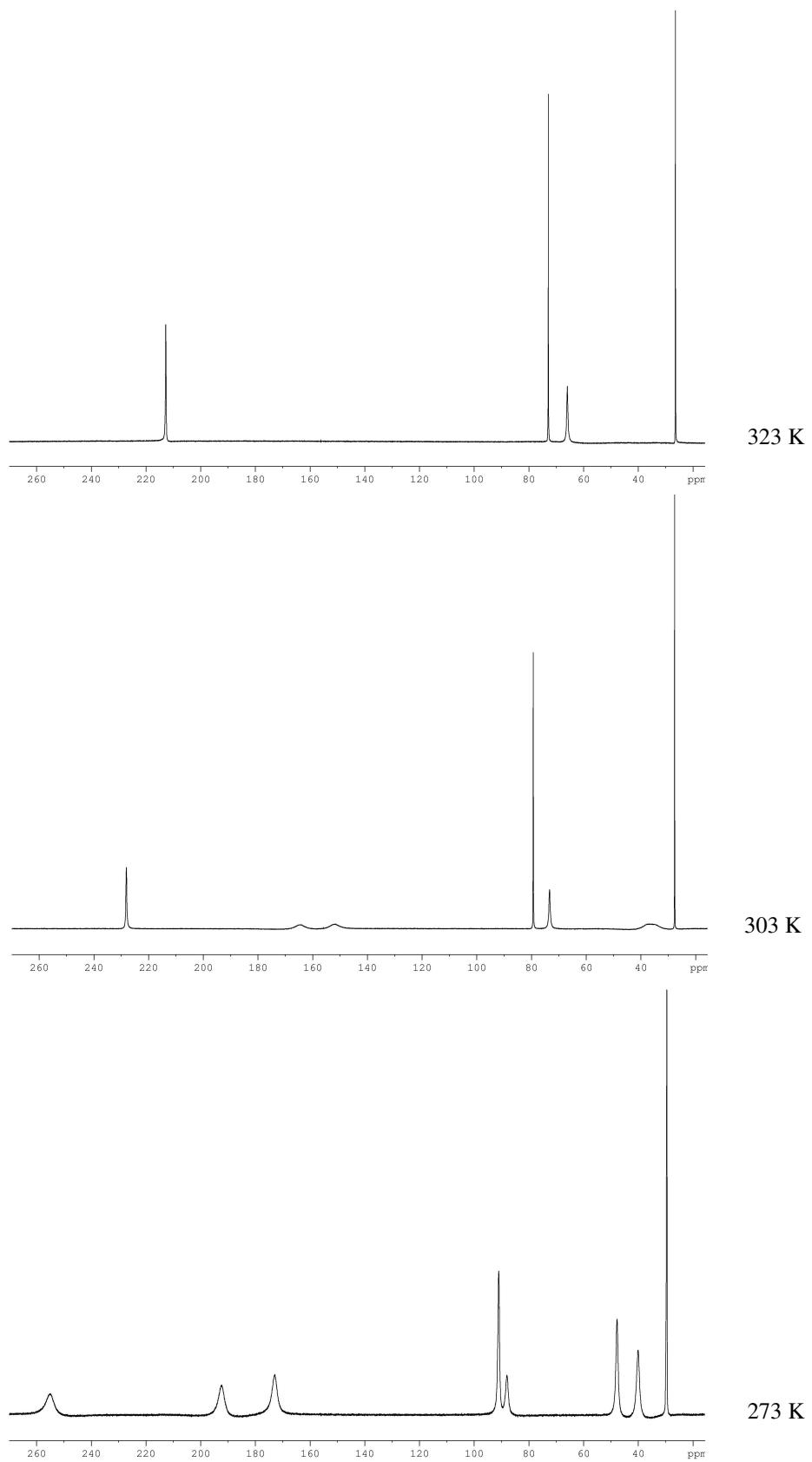
**Figure S4** 500 MHz  $^1\text{H}$  NMR spectra of  $\mathbf{1}[\text{CF}_3\text{SO}_3]_2$  in  $\text{CD}_3\text{NO}_2$  at different temperatures, showing the broadening of the peaks from the diastereotopic ligand methylene groups as the temperature is raised. The variation of the contact shifts of the peaks with temperature is normal, and reflects the decreasing susceptibility  $\chi_M$  of the compound as the temperature is raised. See the main paper for peak assignments.
