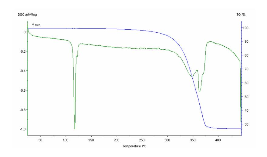
**Figure 2**. TGA/DSC Plot for Zn(TePPr<sup>i</sup><sub>2</sub>NPPr<sup>i</sup><sub>2</sub>)<sub>2</sub> (**6**) [blue: TGA; green: DSC].
