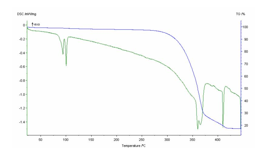
**Figure 4**. TGA/DSC Plot for Hg(TePPr<sup>i</sup><sub>2</sub>NPPr<sup>i</sup><sub>2</sub>)<sub>2</sub> (**8**) [blue: TGA; green: DSC].
