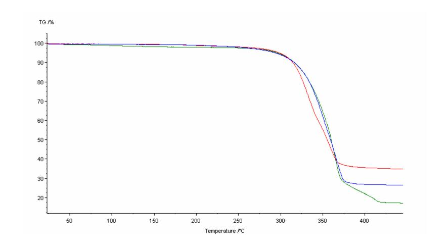
Figure 1. TGA curves for the complexes  $M(\text{TePPr}_2^i\text{NPPr}_2^i)_2$  [blue: M = Zn (6); red: M = Cd (7); green: M = Hg (8)].
