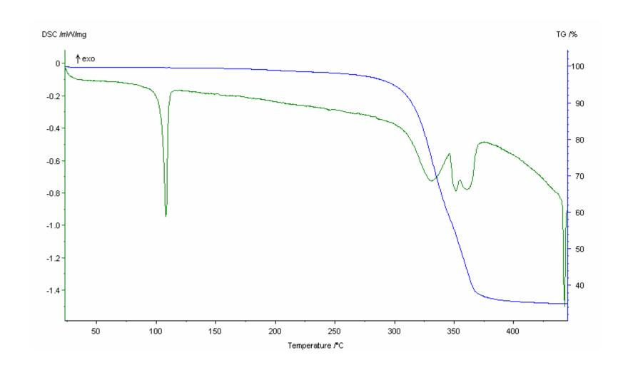
**Figure 3**. TGA/DSC Plot for  $Cd(TePPr_2^iNPPr_2^i)_2$  (7) [blue: TGA; green: DSC].
