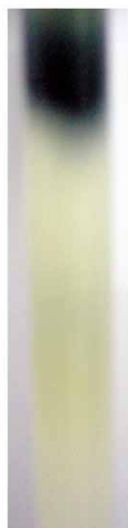
Fig. S5. Photograph of the Sephadex G-50 column. Two distinct colored bands corresponding to [\text{P}_2\text{W}_{15}\text{Mo}_2\text{VO}_{62}]^{8-} (dark blue) and 1 (yellow) have already separated.
