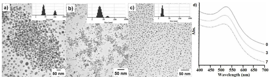
**Figure S8.** TEM images and size distributions (in inset) of Au NPs from  $[\text{C}_{18}\text{-bim}]/[\text{Au}(\text{C}_{18}\text{-bim})_2]\text{[NO}_3]$  with molar ratios of (a) 0, (b) 3, and (c) 7; (d) the corresponding UV-visible absorption spectra for Au NPs obtained at different molar ratios (from top to bottom).
