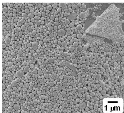
**Figure S9.** SEM image of gold nanomaterials from thermolysis of  $[\text{Au}(\text{C}_{18}\text{-im})_2]\text{[AuCl}_2]$  at 200 °C for 1 h.
