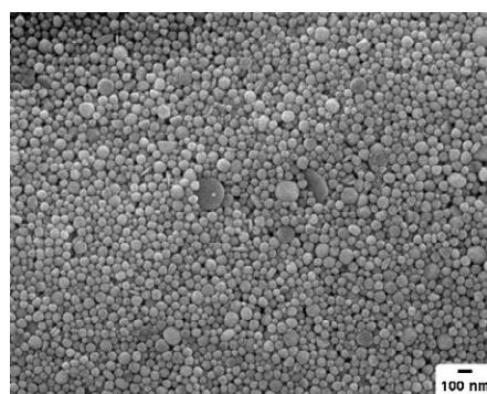
**Figure S12.** SEM image of gold nanomaterials from thermolysis of  $[\text{Au}(\text{C}_{18}\text{-im})_2]\text{[NO}_3]$  at 200 °C (isotropic phase) for 1 h.
