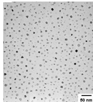
**Figure S11.** TEM images of gold nanomaterials from thermolysis of  $[\text{Au}(\text{C}_{18}\text{-im})_2]\text{[NO}_3]$  at 100 °C (mesophase) for 1 h.
