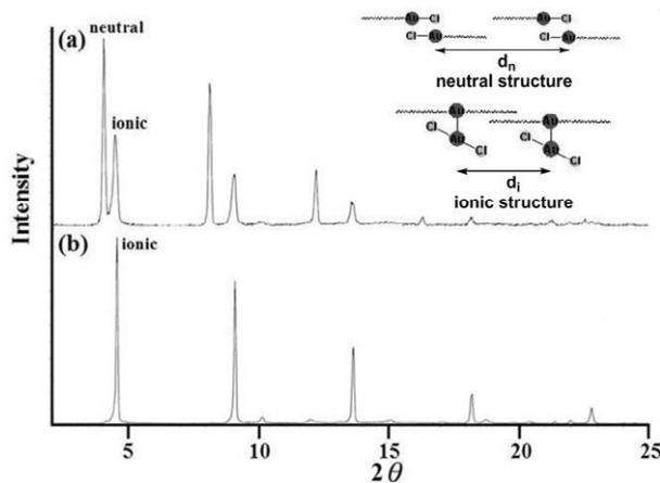
**Figure S6.** XRD diffractograms of  $[\text{Au}(\text{C}_{12}\text{-im})_2]\text{[AuCl}_2\text{]}$ . (a) powder sample obtained by adding hexane to the  $\text{CHCl}_3$  solution, (b) single crystals (ionic compound).
