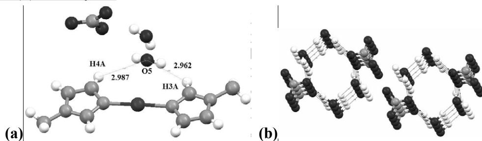
**Figure S4.**  $[\text{Au}(\text{C}_{14}\text{-im})_2]\text{[NO}_3\text{]}\cdot 2\text{H}_2\text{O}$  showing (a) the H-bonding interactions from imidazole, nitrate and water, (b) the hexagon channel formed from nitrate anions and water molecules.
