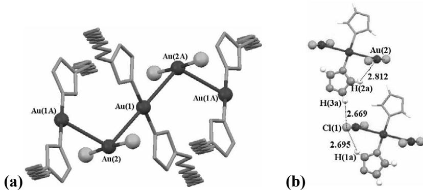
**Figure S2.**  $[\text{Au}(\text{C}_{12}\text{-im})_2][\text{AuCl}_2]$ , (a) the zigzag  $\text{Au}(\text{I})$ - $\text{Au}(\text{I})$  interactions. (b) The C-H...Cl H-Bonding interactions between the cation and anions.
