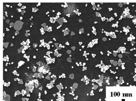
**Figure S10.** SEM image of triangular, hexagonal and spherical gold nanomaterials from thermolysis of  $[\text{Au}(\text{C}_{18}\text{-bim})_2]\text{[NO}_3]$  at 200 °C.
