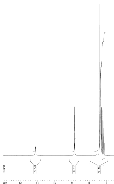
Figure 1 1 H NMR Spectra of 3 in CDCl 3
