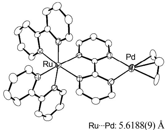
Ortep diagram of the cationic part of **Ru<sup>H</sup>-bpmp-Pd(η<sup>3</sup>-CH<sub>3</sub>CHPh)**.
